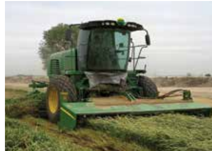
The RCI 316M is available for the John Deere W200 Series (rotary traction unit) self-propelled windrower with a 16 ft. (4.9 m) 995 or 14 ft. 6 in. (4.5 m) 994 Rotary Platform head.
