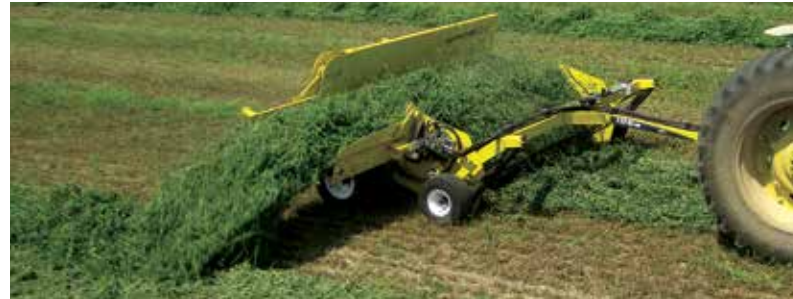
The RCI 186M Merger combines windrows of crop together in preparation for harvest or invert the crop to improve drydown prior to harvest.
