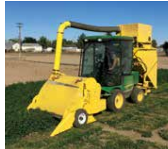
The RCI line of Research Plot Equipment provides for the harvest and sampling of a variety of crops in various conditions.
